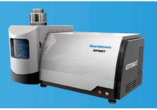
ICP 2060 Sequential Inductively Coupled Plasma Emission Spectrometer is designed to measure major, minor and trace elements in various samples with excellent analytical precision and accuracy. ICP2060 has wide wavelength range of 190nm to 800nm with 2400 line grating. The instrument feature high optical resolution, full automation, Solid State RF system as well as powerful analysis software with auto-matching.
